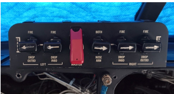
The armament control panel as installed.
