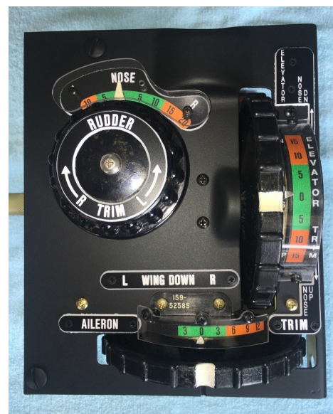
Engine control quadrant before (left) and after (center) assembly. The completed trim control quadrant (right), with its precision indicators.
