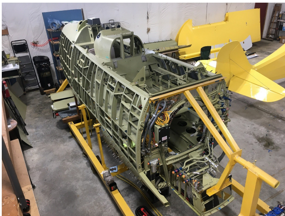
The fuselage structure awaits more skin panels. All photos: Jack LaBounty
