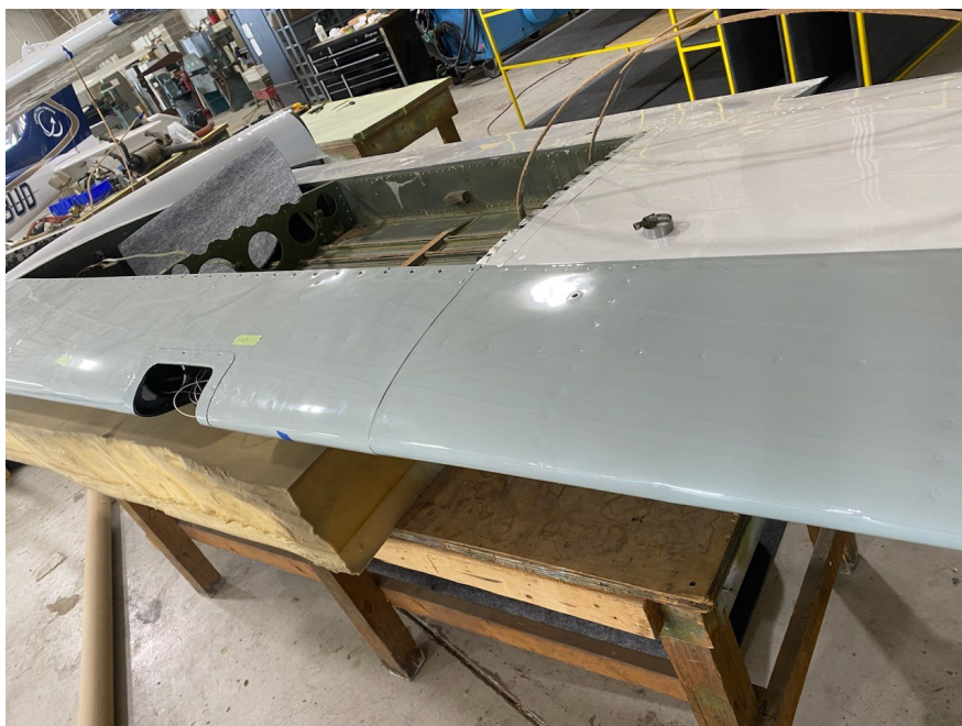
The freshly painted wing being torn apart. The fuel tanks are removed and soon the outboard top skin will be drilled out and replaced.
