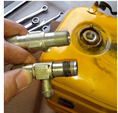
Above: Leaky fuel header tank. Below: New and old fittings.
