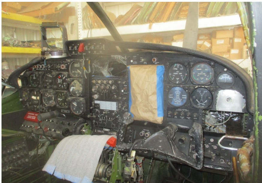
The Electronic Reticle and Armament Control Panel were added to the cockpit. The brown paper covers the faceplates of recently installed radios, to prevent damage.
