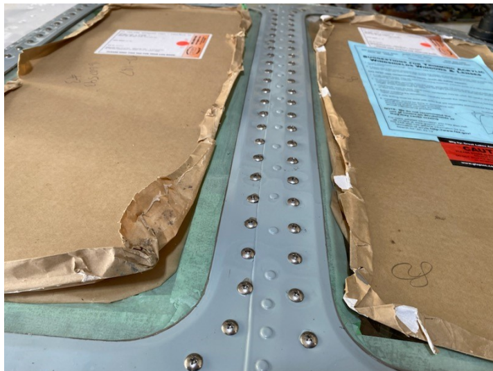
The top windows after replacement. Note the many rivets and screws involved.
