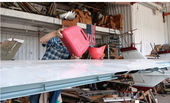
Pouring the first batch of fuel into the right main tank to test the auxiliary fuel pump for the first time. All photos: Jay Borella
