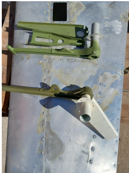
Old, rusty elevator counterweight assemblies were replaced by corrosion-protected new old stock.
