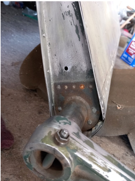
Old, rusty elevator counterweight assemblies were replaced by corrosion-protected new old stock.
