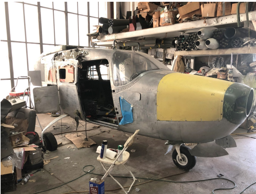
Well into the restoration, getting ready for paint.
