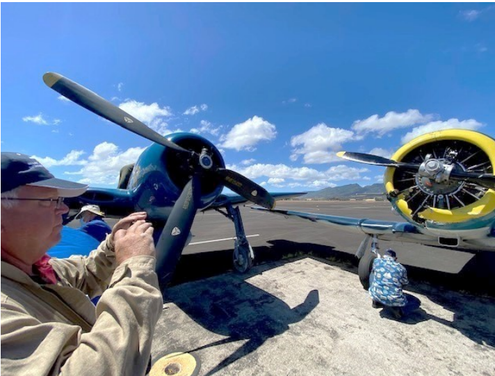
Dave Richardson documents the aftermath of a Bearcat taxiing into a T-6. Note the Bearcat's missing propeller blade and bent tip.
