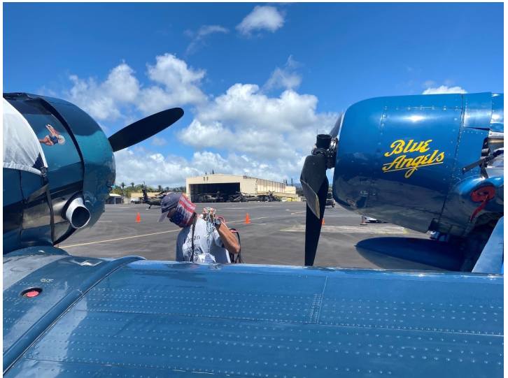
Dave Richardson documents the aftermath of a Bearcat taxiing into a T-6. Note the Bearcat's missing propeller blade and bent tip.
