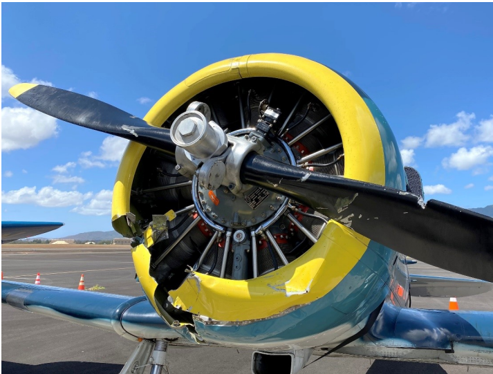
Smokey's T-6 suffered a damaged cowling and propeller, among other less visible problems. Sadly, it sat disassembled for transport during the V-J Day events it was supposed to help commemorate. All photos: John Johnson and Dave Richardson
