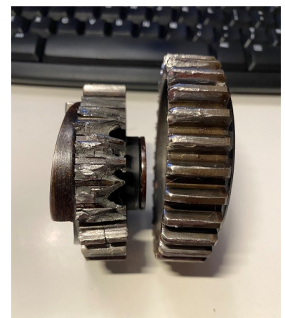
Engine failure culprits—starter gear (left) and crank gear (right).
