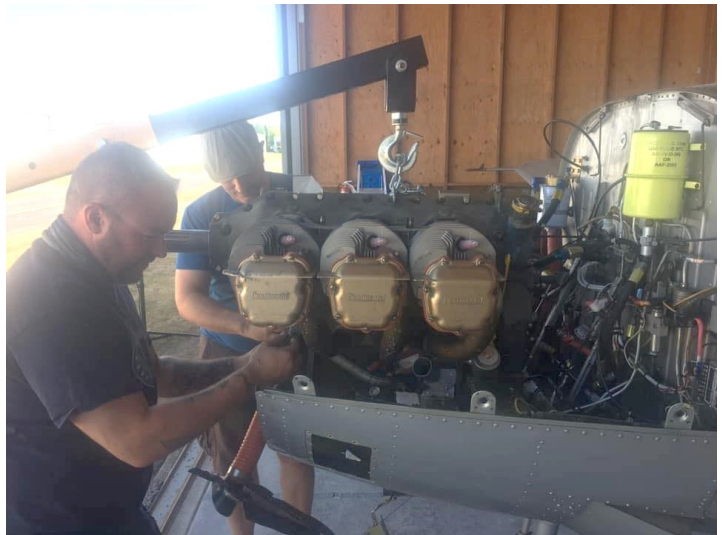
CWB member and Navion owner David Osgood helps new CWB member and Normandy Aircraft owner Logan Shepard install the new engine. Photo: Bill Lattimer
