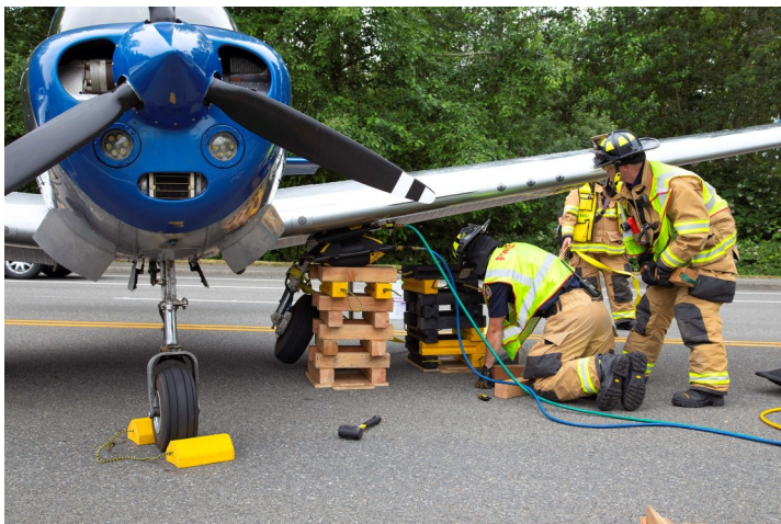
The fire department uses wood blocks and air bags to lift the wing and lock the gear down. Photo: Dan Shoemaker
