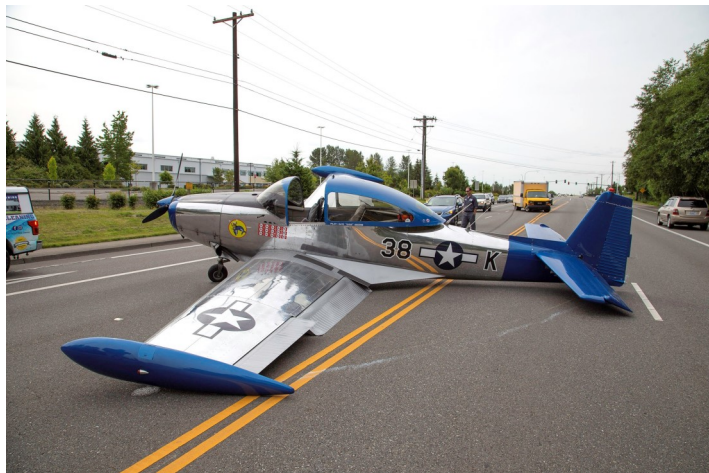
The gear collapse ground down a fuel drain and left a trail of avgas on Airport Road. Photo: Dan Shoemaker
