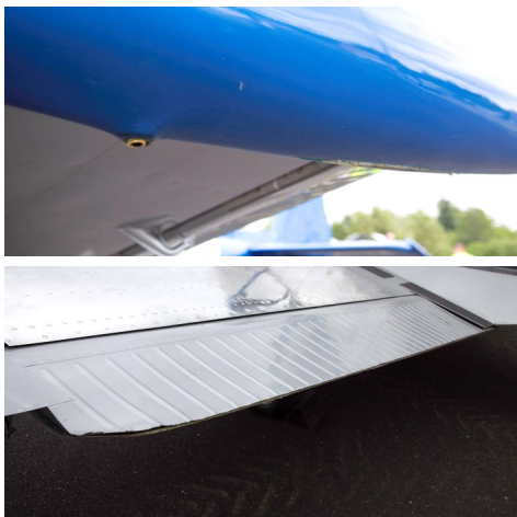
Damage was primarily to a fuel drain, some paint, and a flap. Photo: Dan Shoemaker
