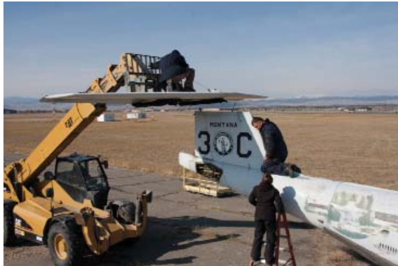
Removing the Horizontal Stab (Lyle Jansma Photo)
