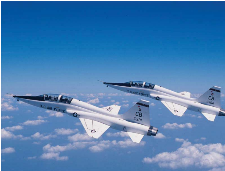
The T-38 Talon, twin-engine, high-altitude, supersonic jet trainer. (U.S. Air Force photo by Staff Sgt. Steve Thurow)
