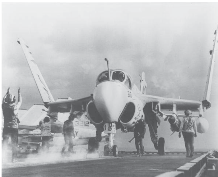
A-6 unfolding its wings as it moves to the cat. (U.S. Navy Photo)
